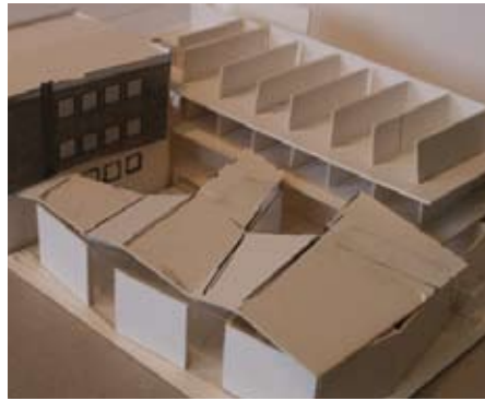
The directions of the wall are broken up and slits are opened up to the street. Attempts with two courtyards, but too narrow. Folded roof in different versions. Roof in two levels to avoid the meeting with the housing volume.
