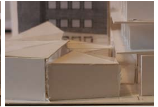
The directions of the wall are broken up and slits are opened up to the street. Attempts with two courtyards, but too narrow. Folded roof in different versions. Roof in two levels to avoid the meeting with the housing volume.
