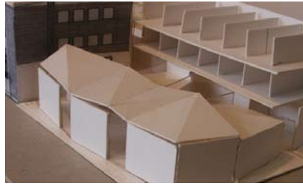
The directions of the wall are broken up and slits are opened up to the street. Attempts with two courtyards, but too narrow. Folded roof in different versions. Roof in two levels to avoid the meeting with the housing volume.
