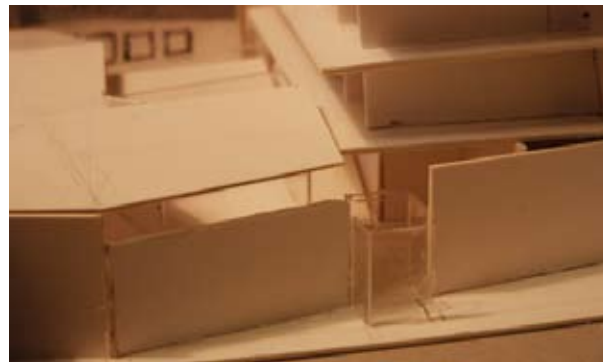
More folded roof in different versions. Roof in two levels to avoid the meeting with the housing volume. Entrance as glass box.
