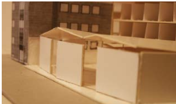
More folded roof in different versions. Roof in two levels to avoid the meeting with the housing volume. Entrance as glass box.
